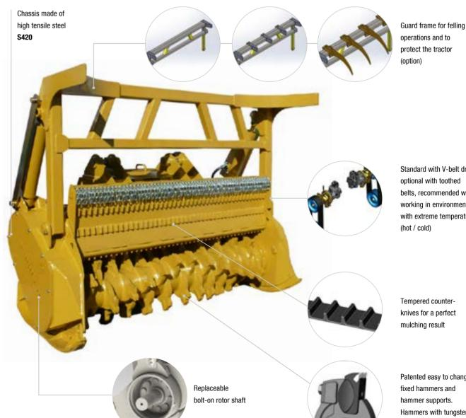
Standard with V-belt drive: optional with toothed belts, recommended when working in environments with extreme temperatures (hot / cold)
