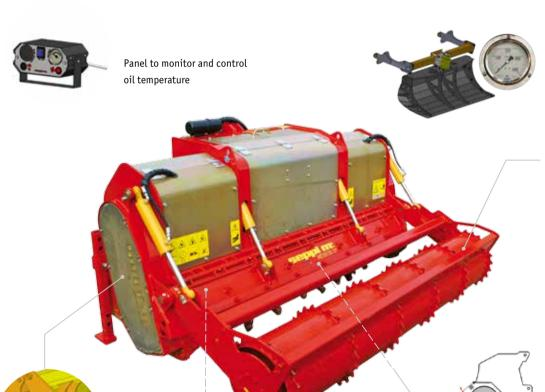
Grader blade (option), hydr. height and rotation adjustment, with hydraulic pneumatic damping incl. lateral extensions · pressure gauge to control work of the grader blade
